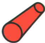
Conical shaped tolerance zone
